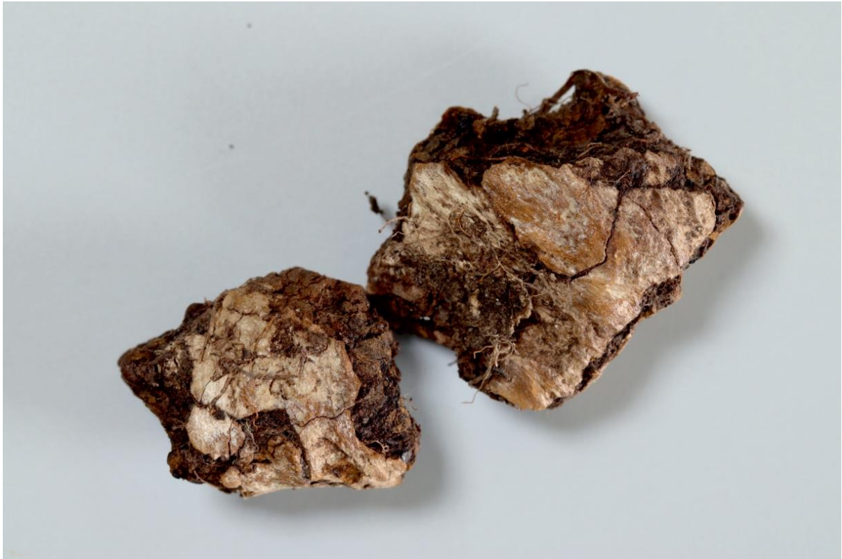
Photo 64. Two fragments of micaceous schist from (102), showing how they are being split apart by the secondary mineral growth. 40mm field of view.
