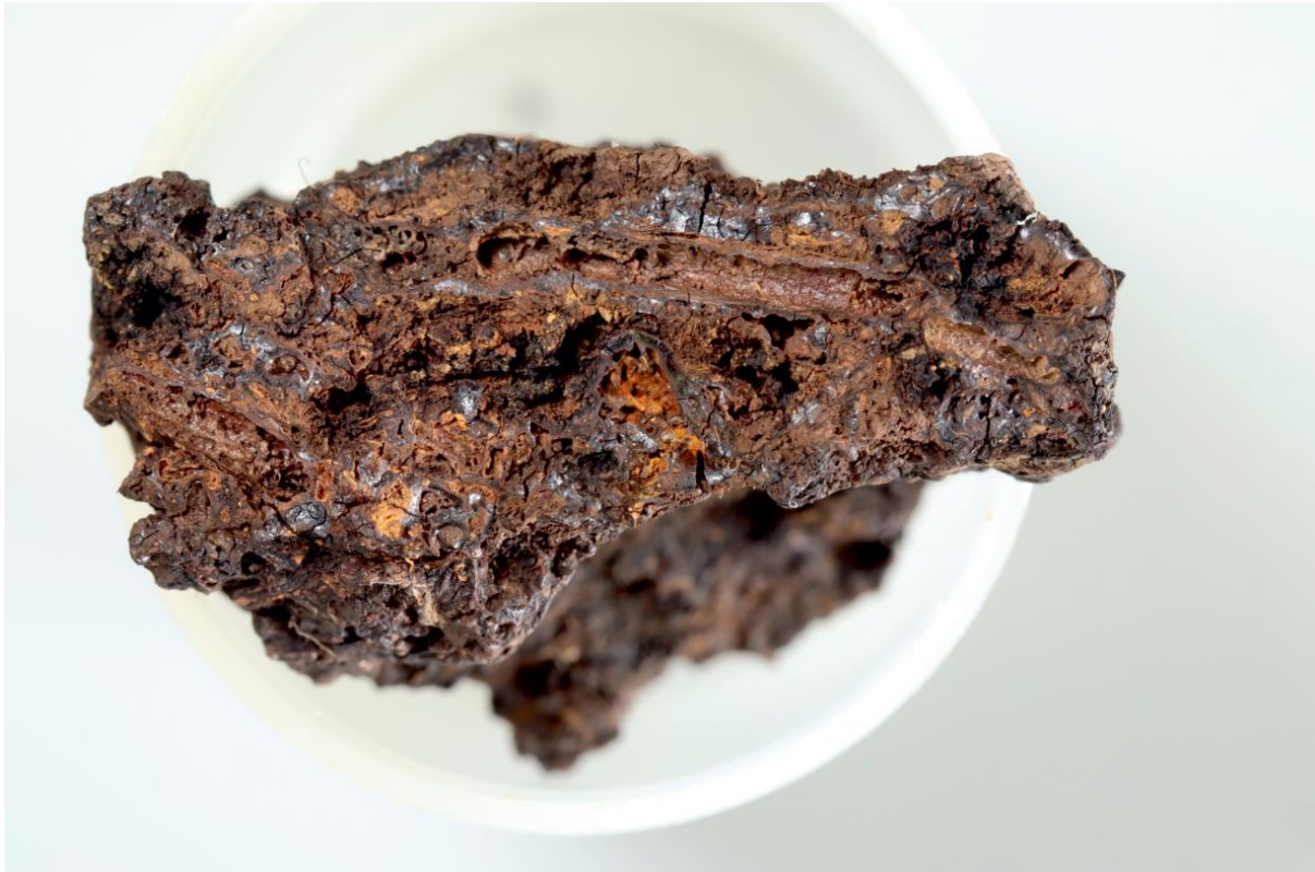
Photo 63. Broken face of an indurated mass from (104). Here the iron enrichment is represented by a very dark brown material forming a sheet-like coating on void surfaces and former organic materials. 40mm field of view.
