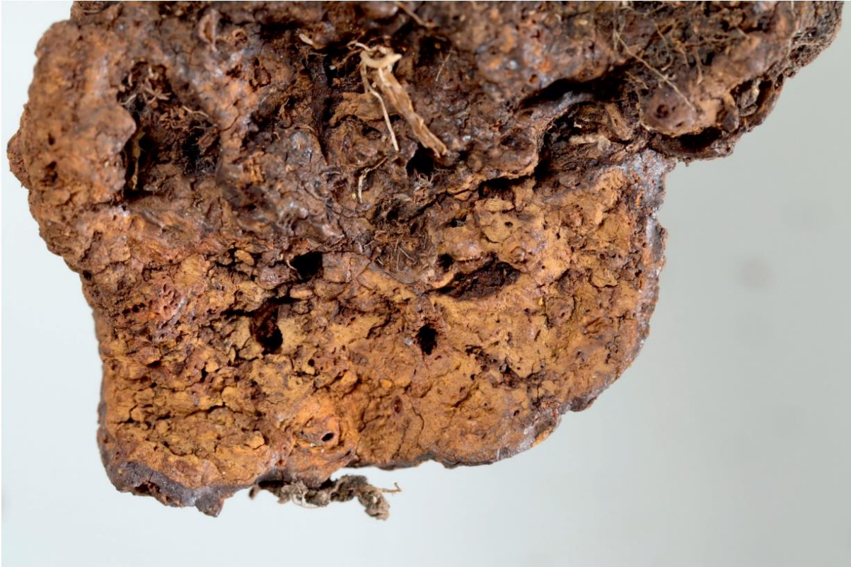
Photo 62. External surface of yellow-brown indurated mass from (102), showing apparent granular texture. 40mm field of view.
