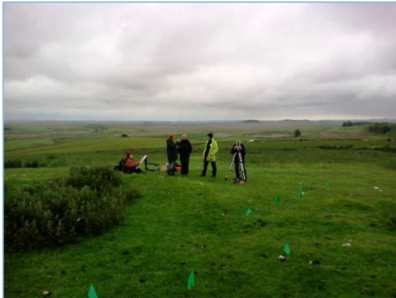
FIGURE 3: THEODOLITE SURVEY OF FLAGGED-OUT ELEMENTS IN AREA 1
