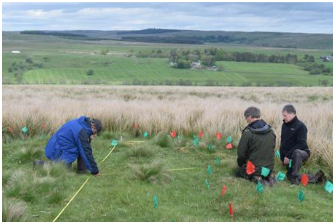
Fig.11 Tape and offset measurement at R09
