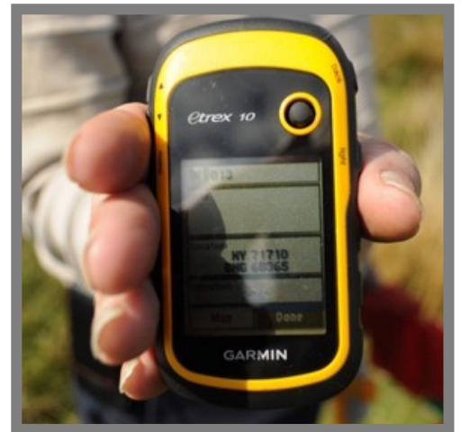
Fig 5.2 Using a hand-held GPS
